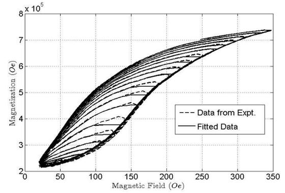
Fig. 3. Results of an identification experiment for a commercial magnetostrictive actuator [20] with a magnetic field discretization of 10 Oe using the maximum negative index method. The results are virtually identical to that obtained using the MatLab<sup>®</sup> function *quadprog* in [5]. See Table IV.
