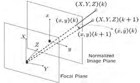
Fig. 3. Object motion in camera frame.
