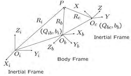
Fig. 1. Kinematics of Camera Motion
