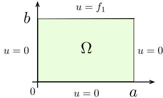
The solution u can be obtained as a sum of the solutions to four simpler problems
