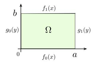
As usual we will start with Dirichlet boundary conditions and a rectangular region  $\Omega$ . The most general setup in this case is to prescribe a function on each of the four sides of the
