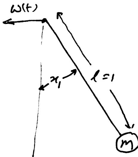
A pendulum is shown in the above figure where the rod has unit length,  $m$  is the mass of the bob,  $x_1(t)$  is the angle of the pendulum from the vertical. We make the usual assumption that the rod is rigid with zero mass and the pivot is frictionless.
