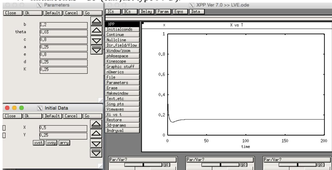
8. In Parameters window change K to 0.5 and hit Go button, change K to 0.75 and hit Go button.
