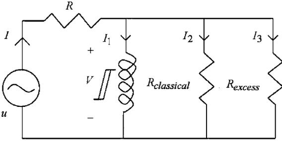
Fig. 1. A magnetostrictive actuator connected to a power supply.
