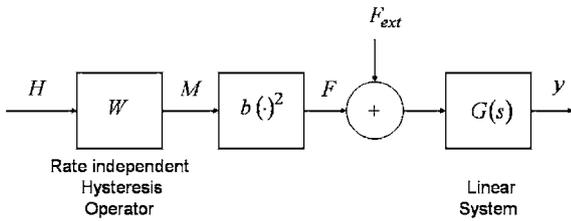
Fig. 2. Model of the transduction of the magnetic field  $H(\cdot)$  to the actuator displacement  $y(\cdot)$ .
