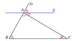
Figure 2.2: The sum of the angles of a triangle is a staight angle
